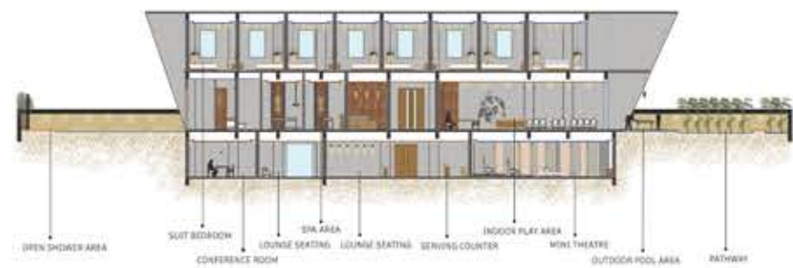
Vertical Sectional Elevation
