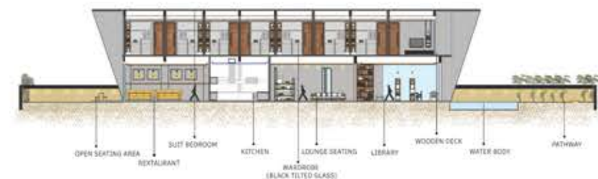
Vertical Sectional Elevation
